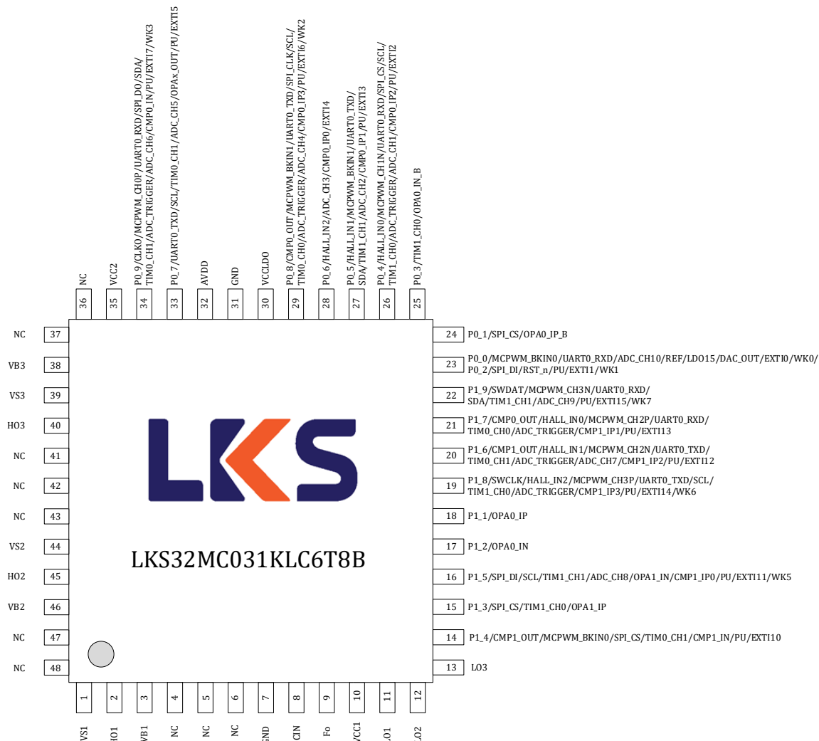
Figure 3-1 LKS32MC031KLC6T8B(C) Pin Assignment Diagram
