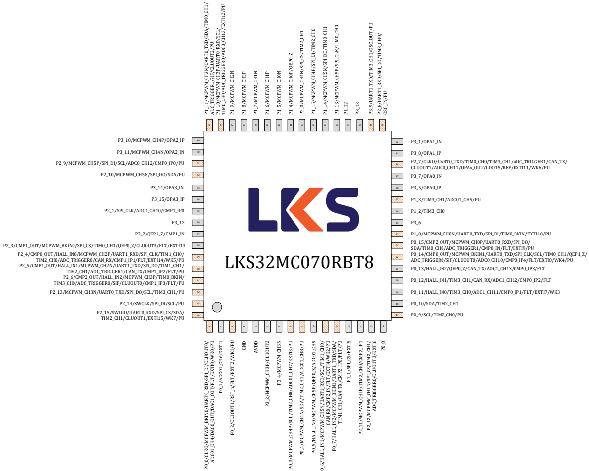
Fig.3-1 LKS32MC070RBT8 Pin Assignment
