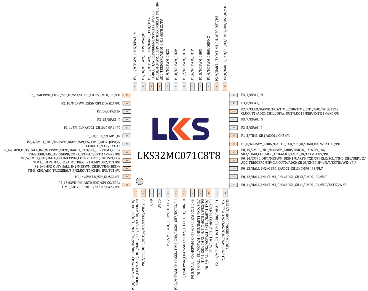
Fig.3-2 LKS32MC071C8T8 Pin Assignment
