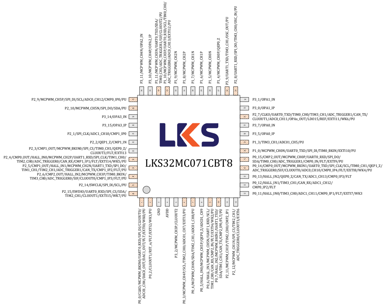
Fig.3-3 LKS32MC071CBT8 Pin Assignment
