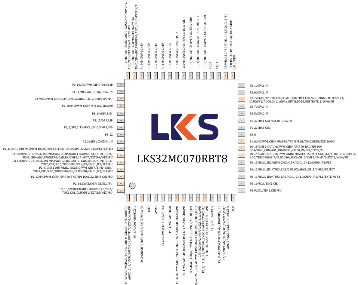
Fig.3-1 LKS32MC070RBT8 Pin Assignment
