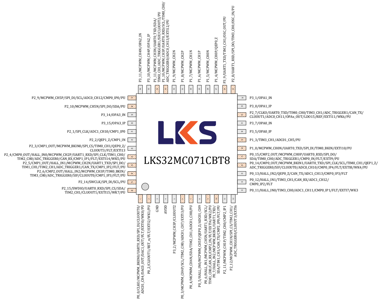
Fig.3-3 LKS32MC071CBT8 Pin Assignment
