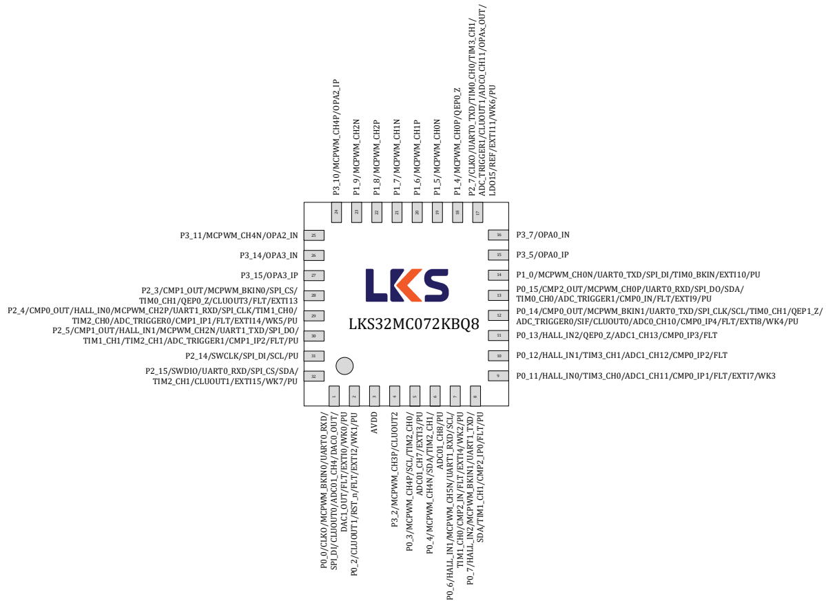
Fig.3-4 LKS32MC072KBQ8 Pin Assignment
