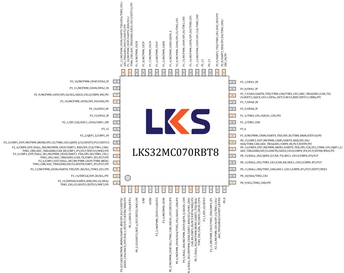
Fig.3-1 LKS32MC070RBT8 Pin Assignment
