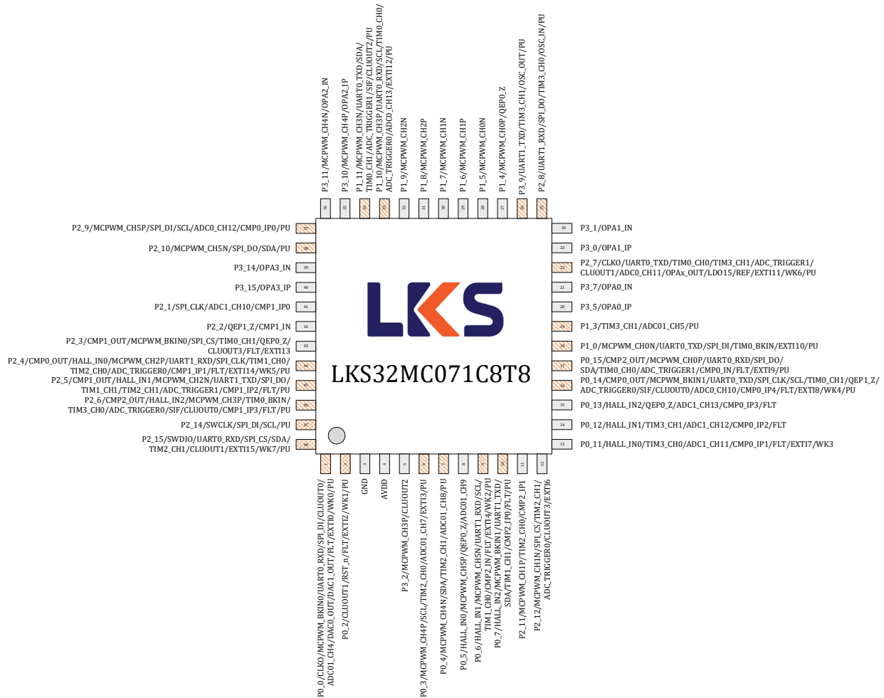
Fig.3-2 LKS32MC071C8T8 Pin Assignment
