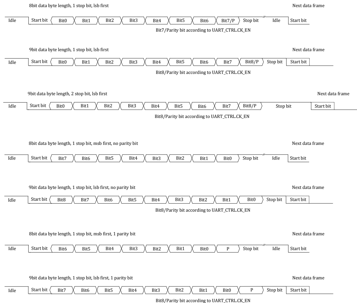
Figure17-2 Uart frame format
