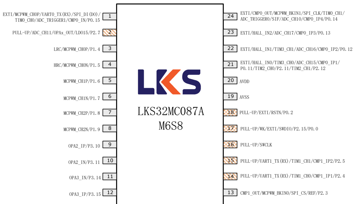
Fig. 3-6 LKS32MC087AM6S8(B) Pin Assignment
