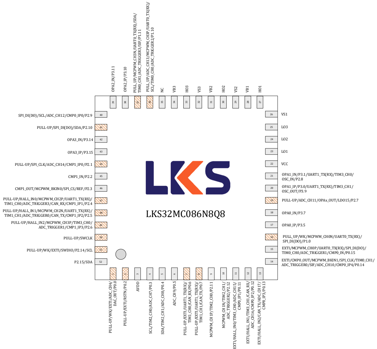
Fig. 3-2 LKS32MC086N8Q8(B) Pin Assignment
