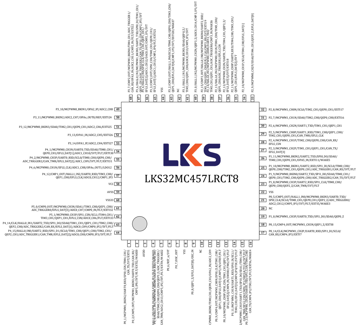
Figure 3-9 LKS32MC457LRCT8 Pin Assignment
