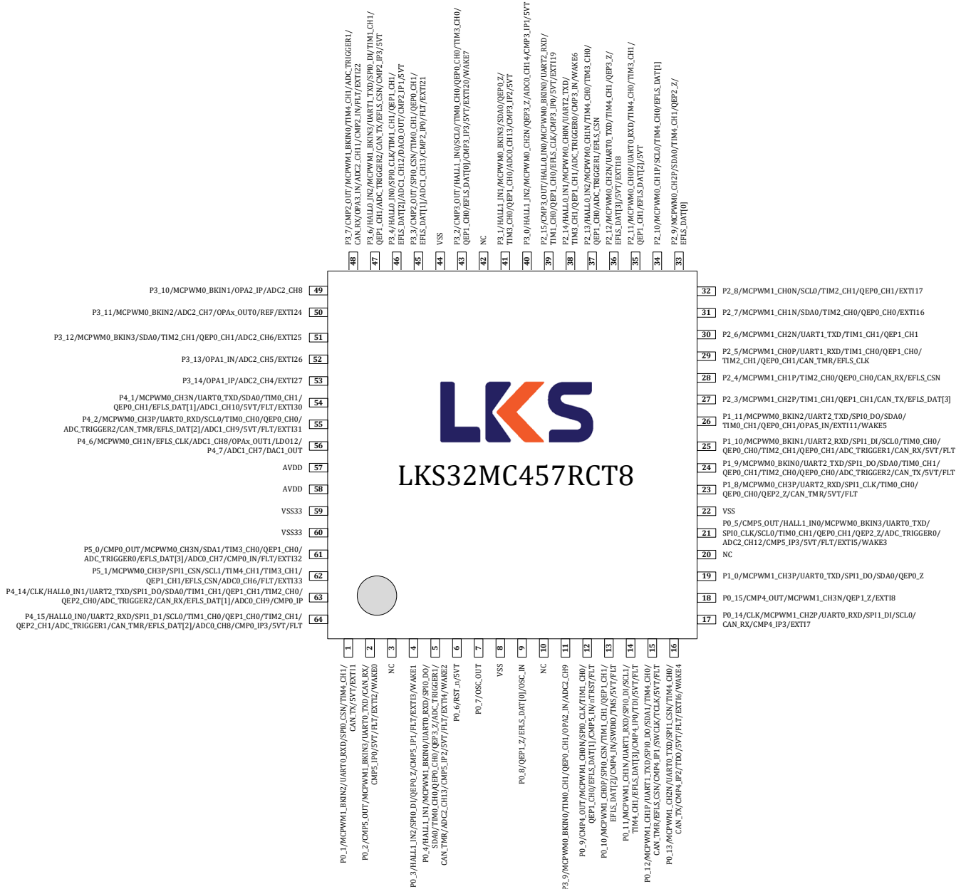
Figure 3-8 LKS32MC457RCT8 Pin Assignment
