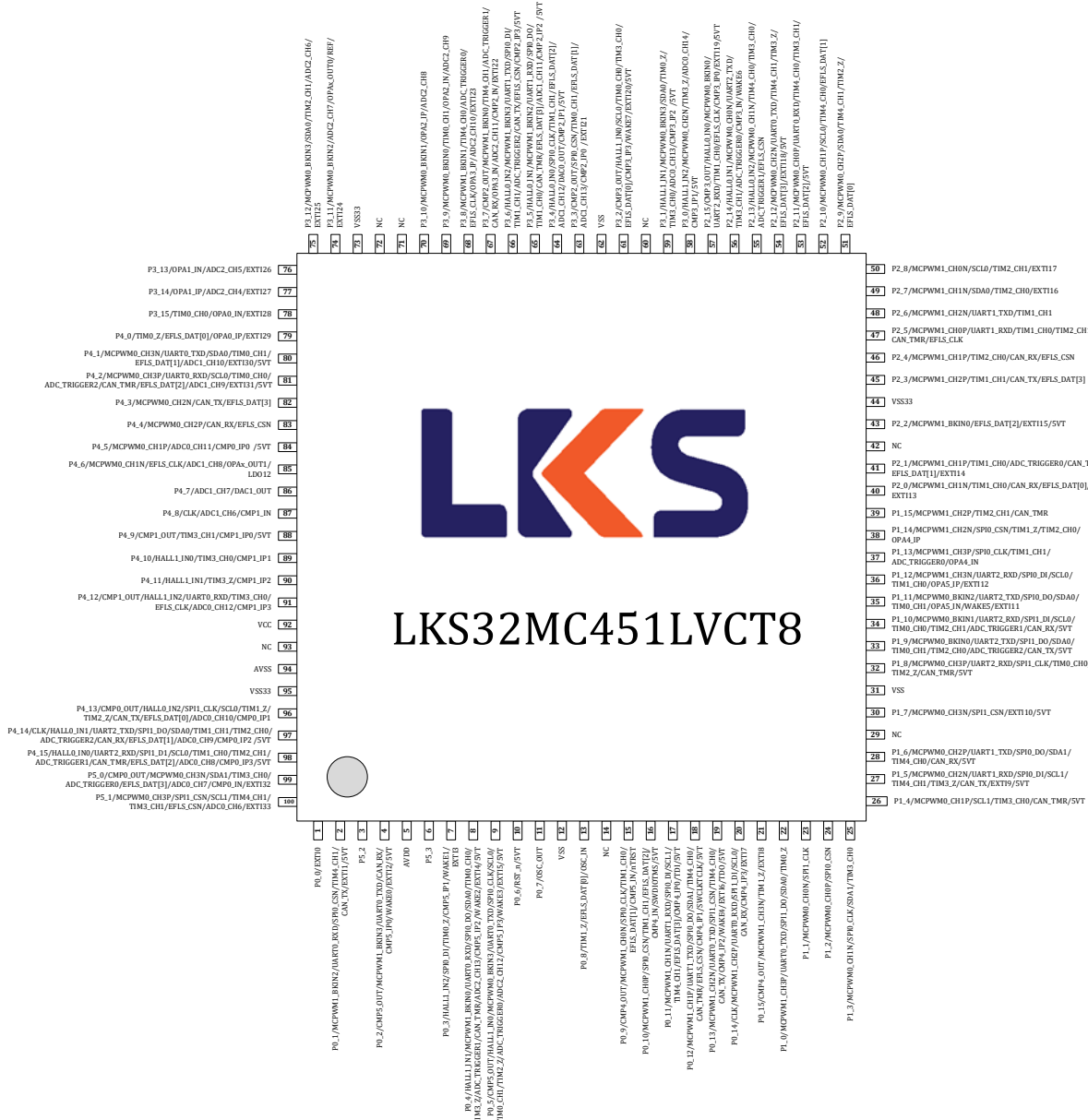
Figure 3-2 LKS32MC451LVCT8 Pin Assignment
