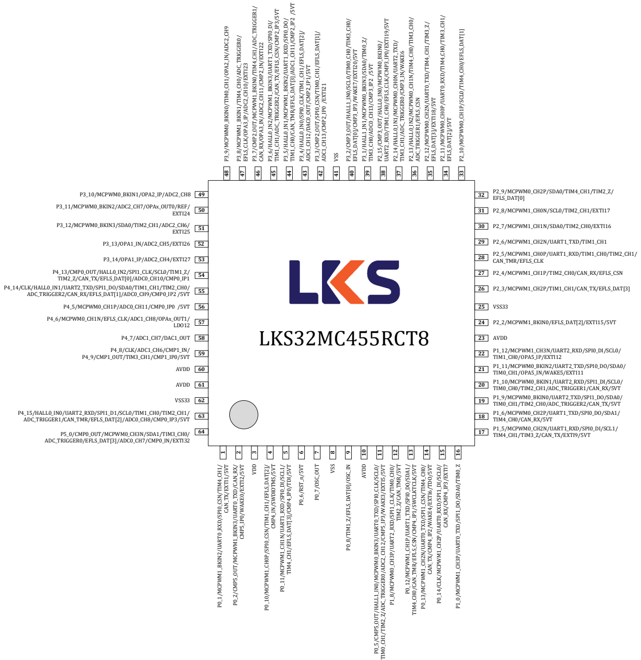
Figure 3-6 LKS32MC455RCT8 Pin Assignment
