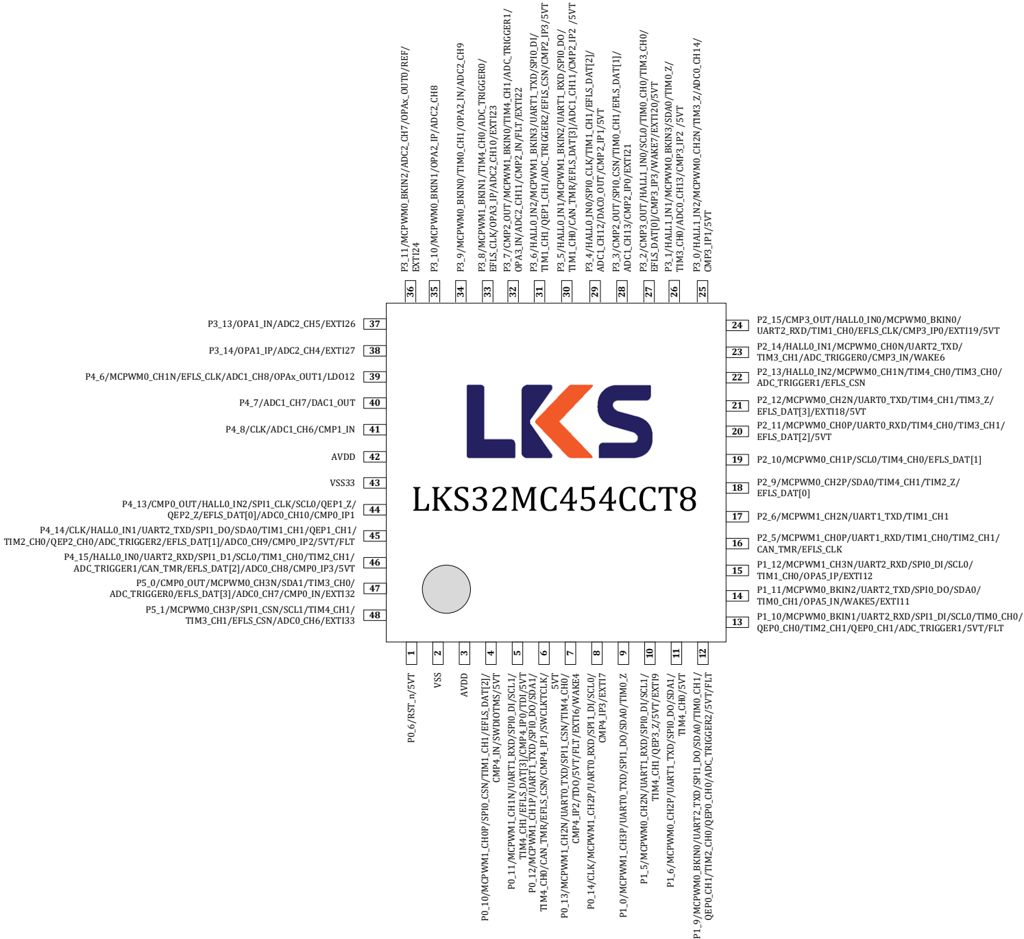
Figure 3-4 LKS32MC454CCT8 Pin Assignment
