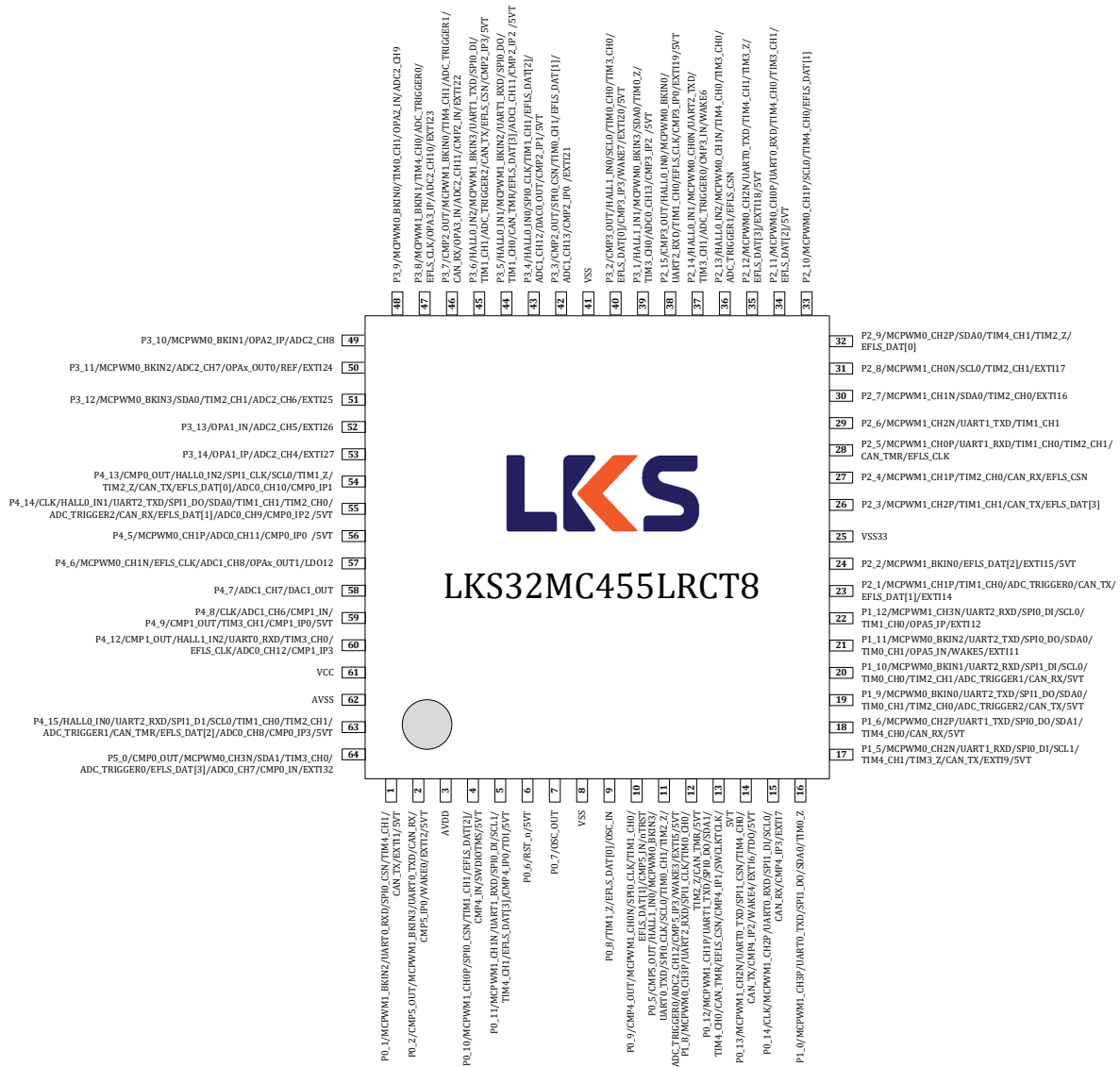
Figure 3-7 LKS32MC455LRCT8 Pin Assignment
