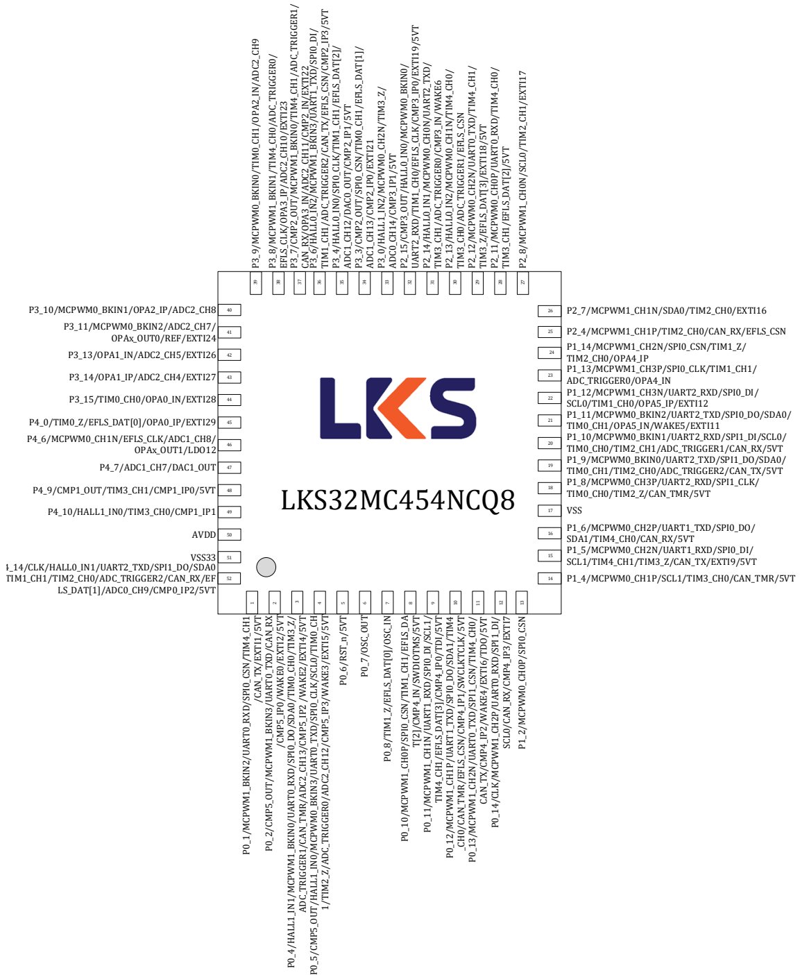
Figure 3-5 LKS32MC454NCQ8 Pin Assignment
