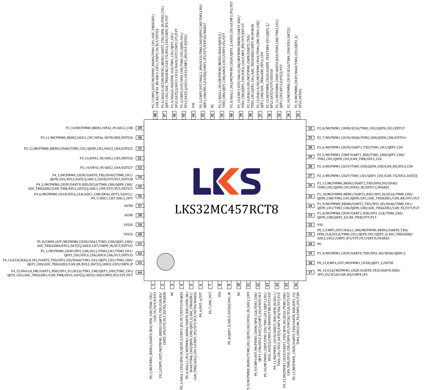
Figure 3-7 LKS32MC457RCT8 Pin Assignment
