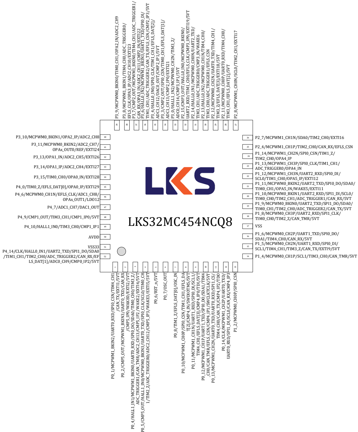
Figure 3-4 LKS32MC454NCQ8 Pin Assignment
