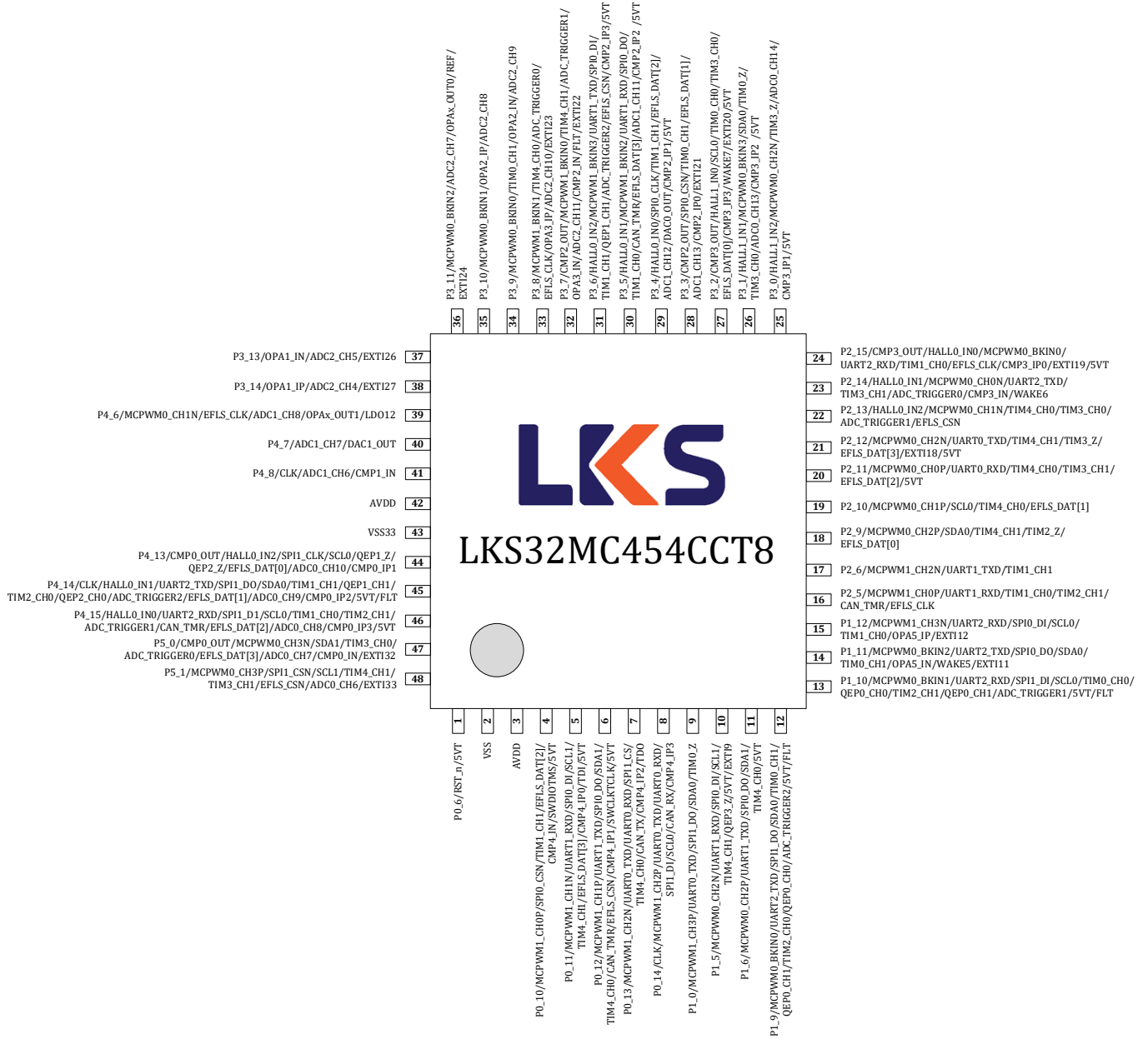
Figure 3-3 LKS32MC454CCT8 Pin Assignment
