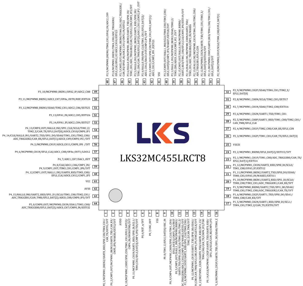
Figure 3-6 LKS32MC455RCT8 Pin Assignment
