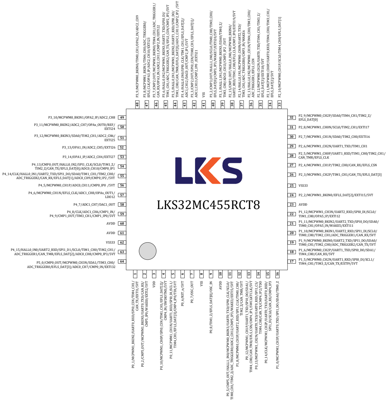
Figure 3-5 LKS32MC455RCT8 Pin Assignment
